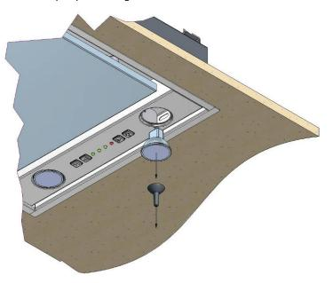
The build-in hood has 2 halogen lights type 12V/20W/Ø35/GU4/38° (reference 7401.029). Total consumption including lights is 210 W for 810/1 - 811, 380 W for 820/1 - 821.
